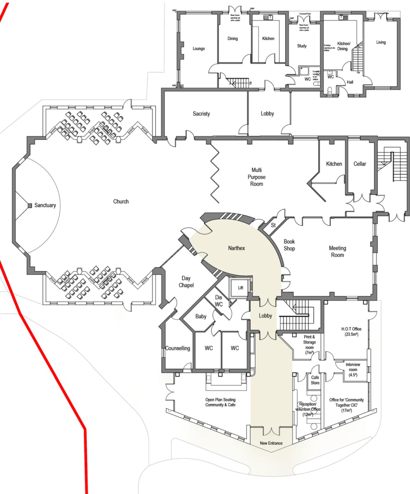
Proposed Ground Floor Plan Scale 1:200
